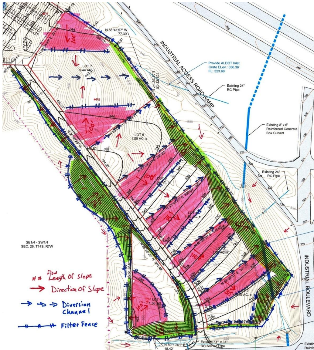
Figure 4-1: Filter Fence and Diversion Ditch Locations
